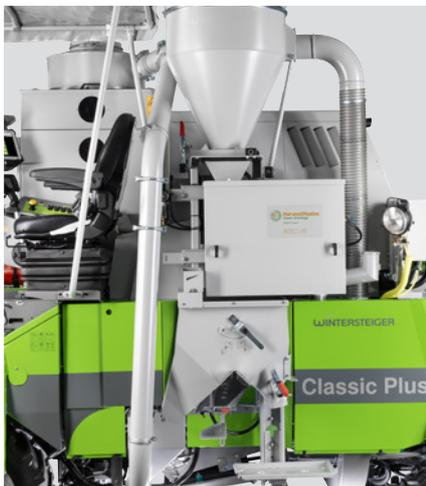
Side mounted sampler (2-man harvesting method)
