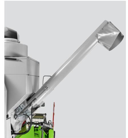
Hydraulic grain tank discharging auger
