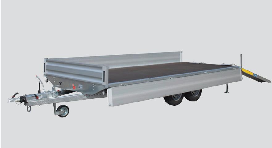
Two aluminum drive-up ramps are stored on the trailer to enable fast loading and unloading. The aluminum side walls with sunk fastenings fold down and are removable. The automatic tow coupling has both an over-run brake and an automatic reverse function.
