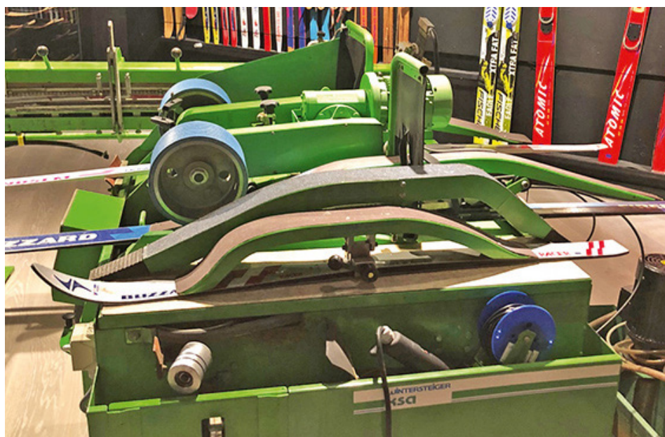
WINTERSTEIGER ski grinding machine MCR 800 (stone, belt and side edge grinder) from 1985. The MCR comes from Solbu Sport in Rauland, Telemark, and was in use from 1985 until Bjarne Solbu closed his shop in 2008. The MCR is still working – just fill it with water and it will be plug and play.
