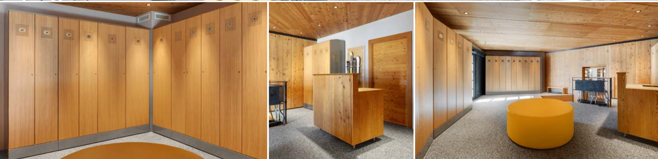
Ski depot in the new five-star Adler Mountain Lodge on the Seiser Alp in Italy. The wooden doors are made of oak wood – three shift glue laminated, brushed and oiled.
