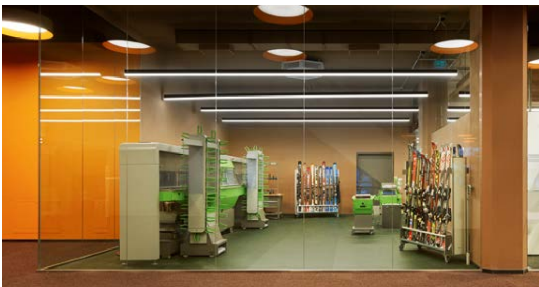
Ski service workshop with Discovery sdp (stone, disc, polishing) fully automatic servicing machine, Sigma Eco belt grinding machine and Waxjet Pro hot waxing machine
