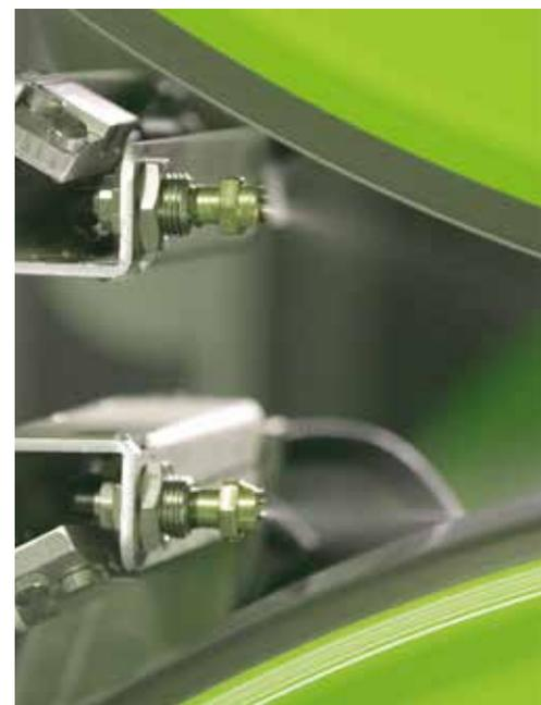
Wet cutting spraying system
