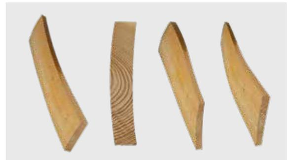
Wooden blocks with longitudinal/latitudinal deformation, cupped or torsion-warped
